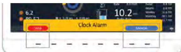
Stop: Press the key on the left to stop the alarm and the alarm will activate again in the next day
